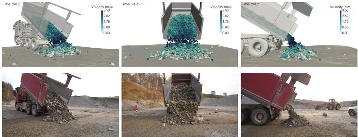
Figure 29. Comparison of C1 aggregate truck experiment and simulation with three different views: ISO, Left, Front displayed at time=24s.
