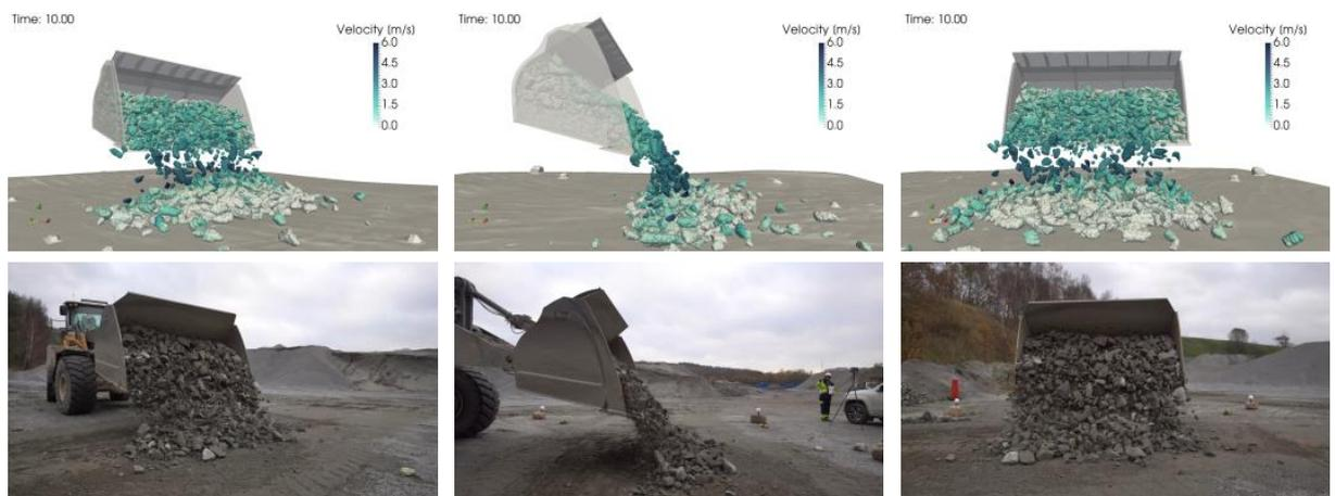
Figure 32. Comparison of C2 wheel loader experiment and simulation with three different views: ISO, Left, Front. displayed at time=10s
