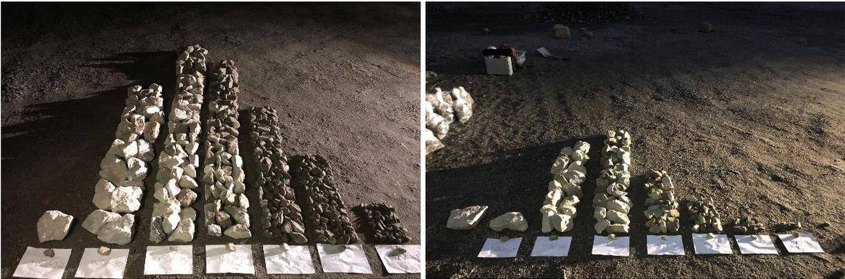
Figure 20. Manually arranged histograms visualizing the size distribution of the +22/-250 mm samples. Left image: C2 Left section. Right image: Front section.
