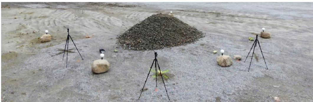
Figure 2. Test area setup (6x6m) in the NCC Stenungsund quarry showing the camera system, 3D scanning reference spheres and the A1 pile formation.
